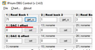
You can set new Register Name, Register Address, Read/Write type of operation and Signed/Unsigned type of read.
