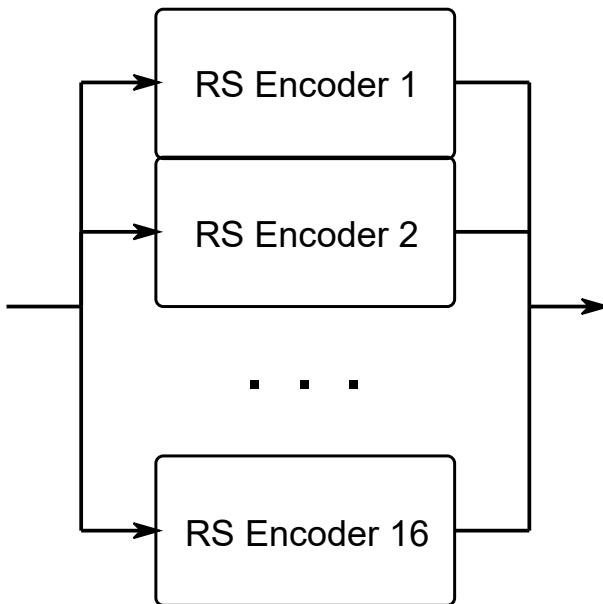
**Figure 1. The G.709 Encoder IP Core block diagram**
