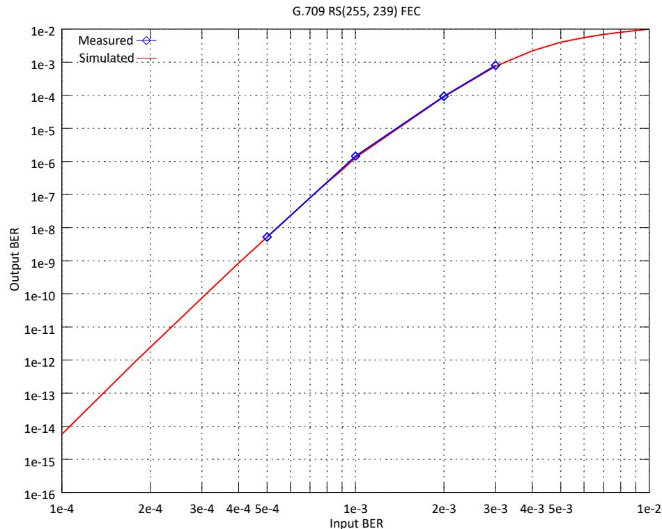
Figure 6. The error-correcting capability of the G.709 Codec
