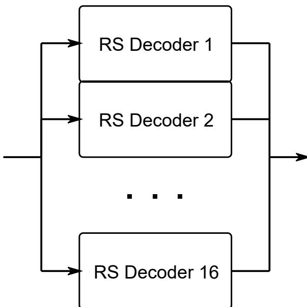
**Figure 2. The G.709 Decoder IP Core block diagram**
