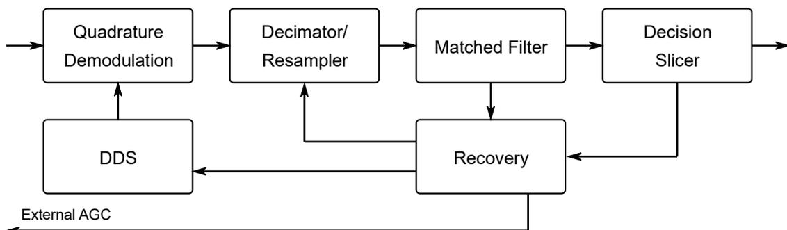
**Figure 1. The QAM Demodulator IP Core block diagram**
