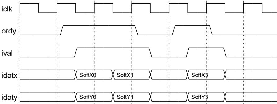
Figure 3. The Viterbi Decoder input timing diagram
