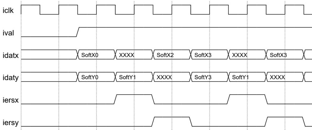
Figure 5. The Viterbi Decoder depuncturing timing diagram
