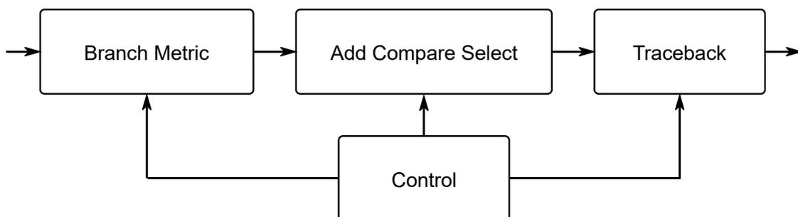
**Figure 1. The Viterbi Decoder IP Core block diagram**
