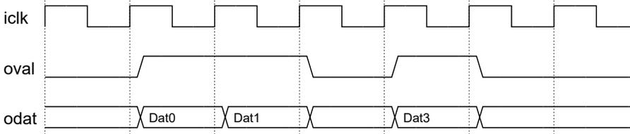
Figure 4. The Viterbi Decoder output timing diagram
