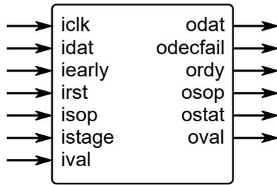
**Figure 4. The LDPC NASA Decoder port map**
