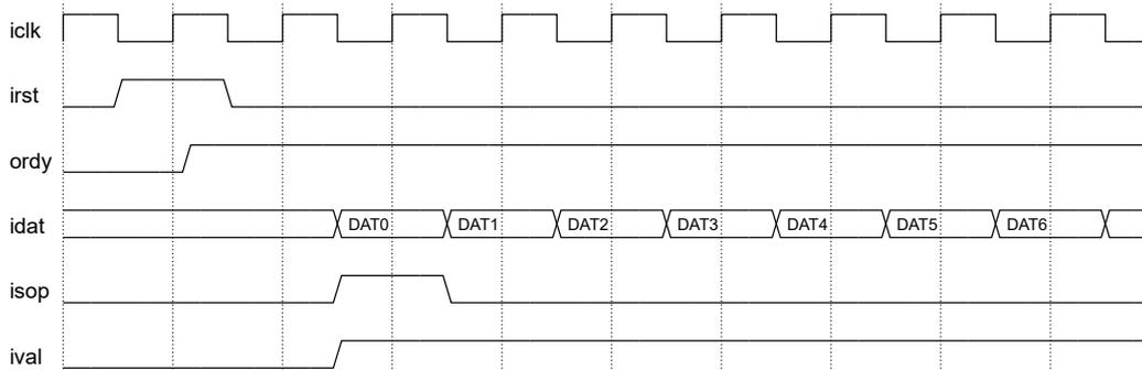
Figure 5. The timing diagrams of the LDPC NASA Decoder operation (input)
